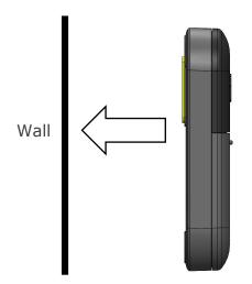
iii> If move in the direction of the arrow,the Bracket will be attached to the wall.The remote is can magnetically attached and detachable.
