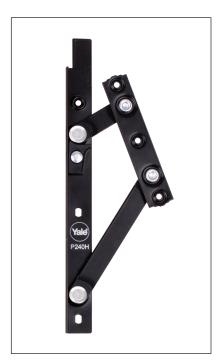
Developed in response to changing market requirements for larger window sashes in projected top hung (PTH) windows, the Nexus range can support window weights of up to 60kg and 2m in height, while still maintaining endurance performance and handle forces, making it the highest capacity aluminium residential window stay on the market.
