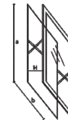
Sliding windows set on side walls Effective area of smoke exhaust window S=1/4 \times (2a+2b) \times H and S \leq a \times b
